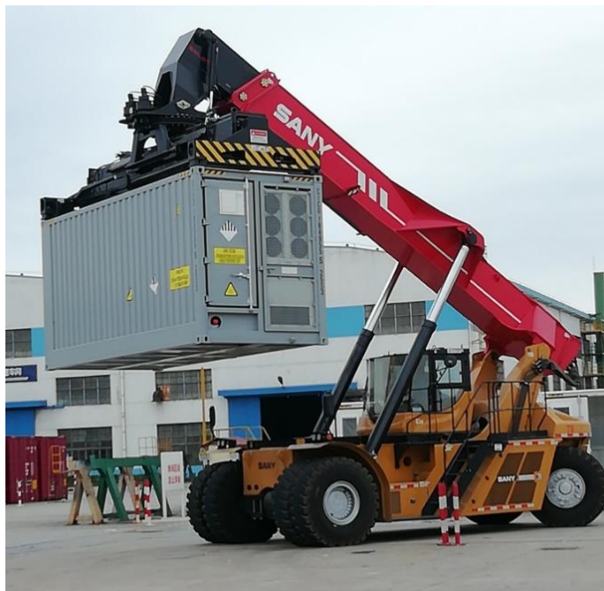
Figure 4-3 Top lifting by four points vertical crane
