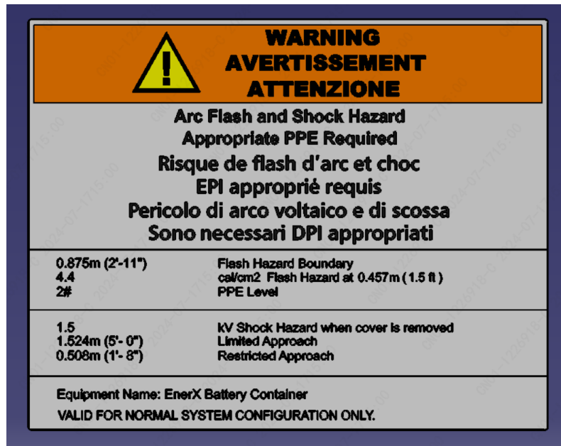
Figure 1-2 Arc Flash Label
